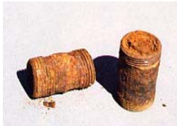
IRON PIPE NIPPLES CORRODED, FILLED WITH RUST AND SLUDGE
